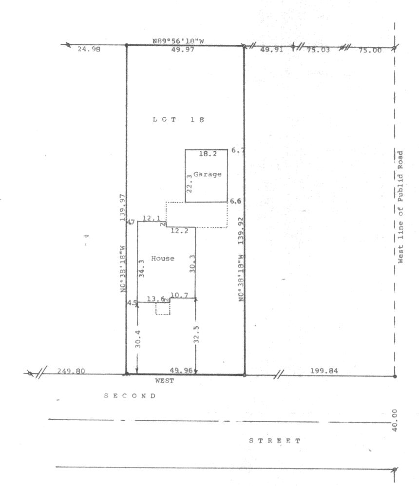
Scale -1'' = 20'# = 14" Iron Pipe Found X = 1" Iron Pipe Found  $\phi = \frac{1}{2}$ " Iron Pipe Found •= 3/4" Iron Pipe Set o = 1" X 24" Iron Pipe Set Bearings referenced to the north line of Second Street with the assumed bearing of WEST. Survey ordered by: Realty World, Carmin Realtors
